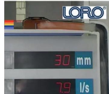
The suction effect of the downpipe propagates throughout the closed siphonic flow system as far as the drain and provides for a strong discharge from the roof.
