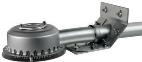
The patented suction cover enables a controlled water/air mixture that minimises cavitation and noise development.
